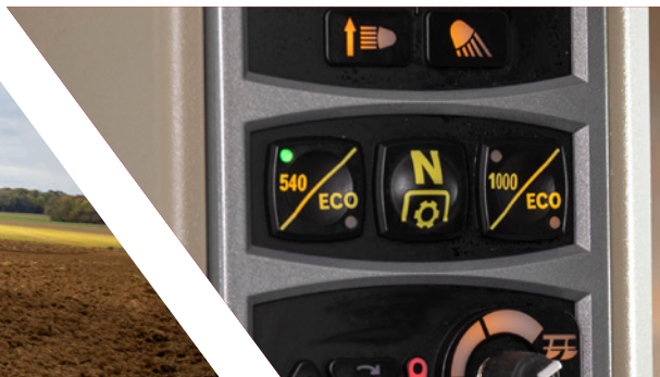
Electro-hydraulic PTO speed selection
