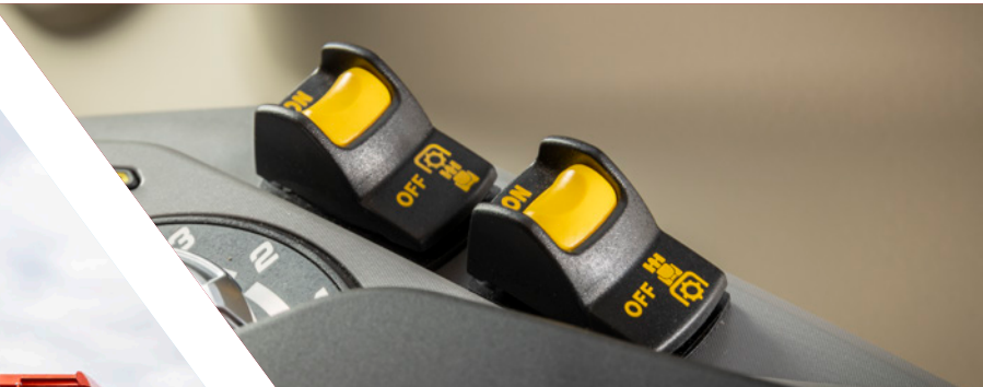
Electro-hydraulic PTO speed selection
